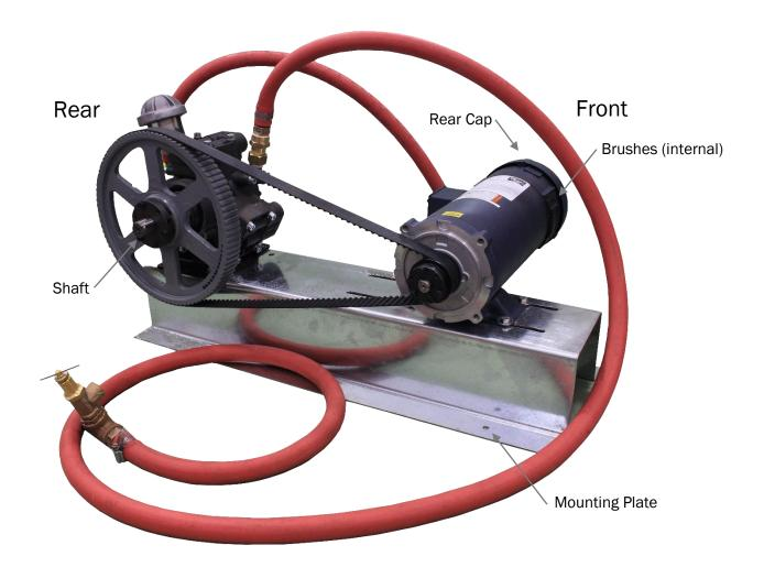
The above displayed SolarRam model is shown without a belt guard for illustration purposes.
