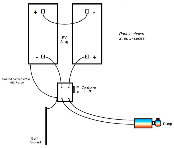
Figure 6-1: System Wiring for Typical PV-Direct SlowPump Installation
