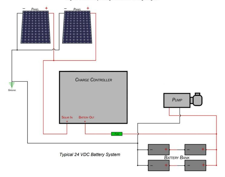
Figure 7-1: Battery Charge Controller Wiring Diagram
