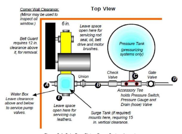
Figure 2.1: SolarRam Piston Pump System Layout
